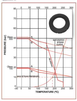
A = Carbon Steel Body Rating, B = Stainless Steel Body Rating (in accordance with ASME B 16.34)
